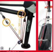
Cunningham Downhaul System/Boom Vang A) Add to the existing Cunningham Downhaul System: 2 x extra single pulley + extra rope 45 cm length. Cunningham downhaul rope lengthened to have a total length of 360 cm (320 cm original + 45 cm extra). Rig the system as shown in the photo to give an extra 2 pulleys leverage on the Cunningham system.
