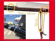
Outhaul and Top Mainsheet Pulley Lower the top mainsheet pulley with an extra rope, Maximum lenght = 20 cm-
